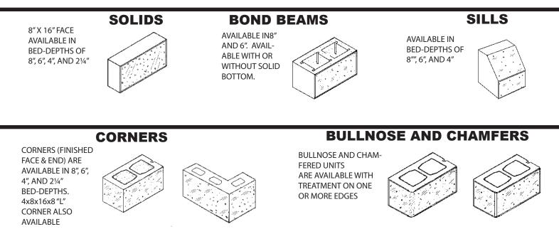
DILLON IS A CUSTOM DESIGN ACMU MANUFACTURER. WE BUILD OUR BLOCK TO YOUR SPECIFICATIONS. OUR SELECTION IS VIRTUALLY ENDLESS FOR CUSTOM SIZE, SHAPE OR COLOR. ALL BLOCK MEET OR EXCEED ASTM OR BUILDING CODE STANDARDS. FULL SIZE SAMPLES AND COLOR SELECTION KITS ARE AVAILABLE UPON REQUEST. DETAILED SPECIFICATIONS ARE AVAILABLE FOR DOWNLOAD.
