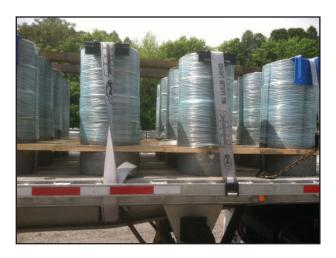
CribPac<sup>™</sup> is a patented system designed using steel fiber reinforced donut crib blocks in 4, 5, & 6 layer
